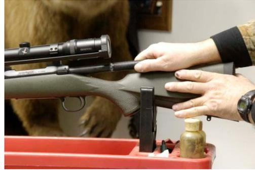
set the rifle up in a cleaning cradle or lightly clamp it in a padded vise to hold the rifle steady. Select the appropriate bore guide for that individual rifle and insert the bore guide in the action insuring it is positioned in its full forward position. Select the appropriate sized cleaning rod and a patch that will snugly fit the bore (for instance I use a 30 cal jag and 2 inch round
