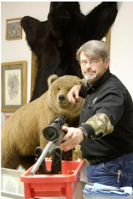
A cleaning stand should be used to steady the rifle and position it so that the rod can be easily guided through the bore in a straight manner. A cleaning stand is illustrated here with a custom hunting rifle mounted in it. Notice the bore guide that has been inserted into the action to help guide the cleaning rod. Try to position the cleaning stand high enough and at an angle that lets you easily guide the cleaning rod without bending or bowing it.
