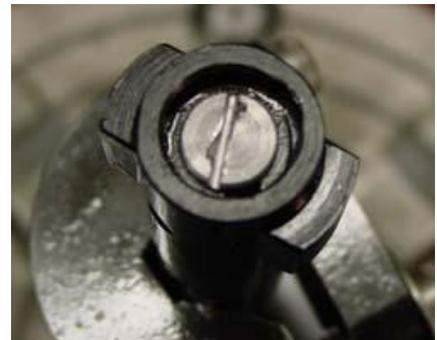
Figure 2—Custom made screw in place and ready to machine
