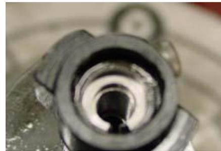
Figure 1-Remington Boltface with holes and counterbores machined
